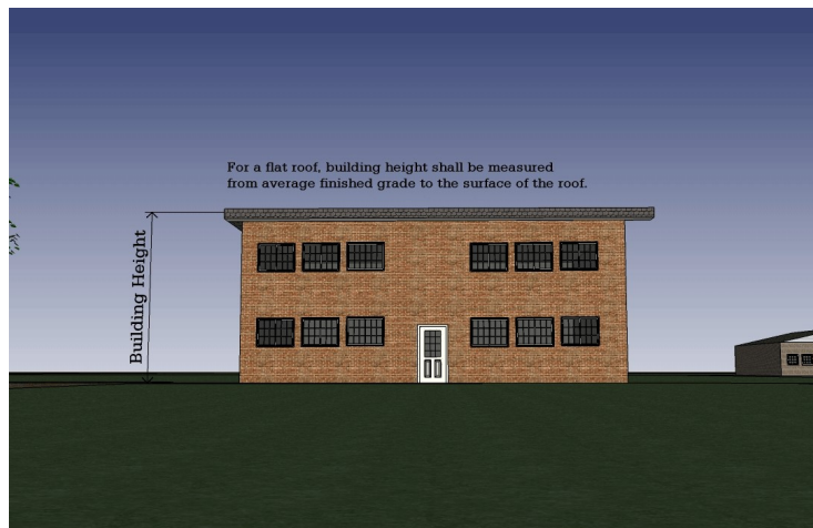
Figure 3.13: Height (Flat Roof)
